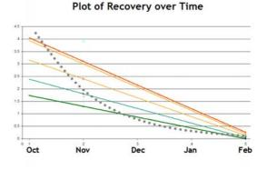
By adding ground movement profiles over time using the level data from the site of the Aldenham Willow we see how much movement takes place over time, and from this tree, on this site at this time, plotting month by month movement with the lowest profile recording the September profile.
