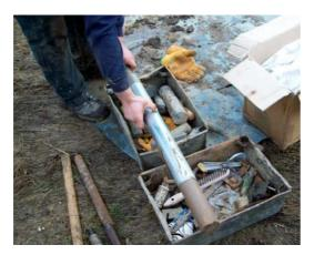
Picture of the tubes and core using a top driven hydraulic jack hammer.
