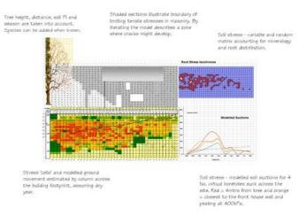
The system works very well on outcropping London clay. The model has an empirical base, using claims data gathered from this location so a degree of success would be expected.
