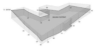
Above is a 3D distortion profile relating to readings taken in October, 2009. Below is the plot of the speed of recovery over time using linear trendlines.
