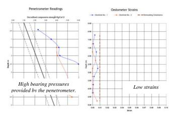
Penetrometer (left) and oedometer results from the same site in Kent, showing very different results. The high penetrometer values are associated with the overconsolidated clay and are not indicative of root induced desiccation, as confirmed by the oedometer, there is negligible swell potential, and no evidence of desiccation.
