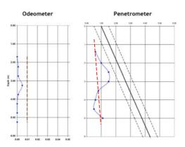
Similar profiles. Note the apparent need to adjust the equilibrium line (suggested by the red dotted line) in the penetrometer graph. The penetrometer appears to detect the low strains recorded by the oedometer.
