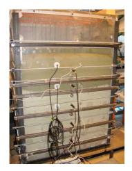
They instrumented a tank with RH and Echo sensors, tensiometers and psychrometers to compare results, and found "the response of the TP sensor has been found to be in agreement with that of suction measurement, while the response of the ECH2O-TE showed some anomalies".
