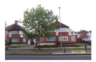
The street-scene doesn't appear particularly threatening at first sight. The tree has a relatively sparse canopy with a sensible distance between the tree and building, and a lawn – room for rehydration in the winter. The front gardens haven't been concreted over to make a car parking space.
